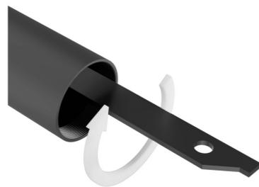
A wire brush with softer wires can be used to clean threads and less dirty parts. The baffle assembly is made of high strength steel and then the surface is nitrided. It can therefore withstand the somewhat coarser cleaning method of a wire brush. It can also be cleaned with an ultrasonic cleaner. After cleaning, dry all components and treat the steel ones with a suitable preservative, e.g. CLP
